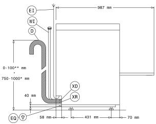
Drain ΕI Electrical inlet (power)
